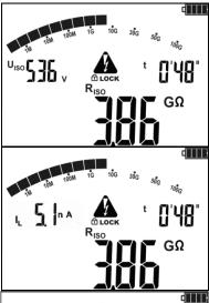
Use **SET/SEL** to display values of leakage current I<sub>L</sub>.
