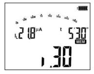
The value of leakage current  $I_L$  measured in time t=5'30'. Symbol  $J_{\rm s}^{\rm M}$  indicates the selected time interval, in which the leakage current value was recorded.
