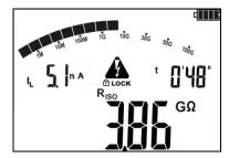
Use **SET/SEL** to display values of leakage current I<sub>L</sub>.
