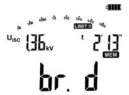
If the electric resistance strength of the tested insulation is exceeded and the puncture occurs, the main field of the display will show message br. d - breakdown
