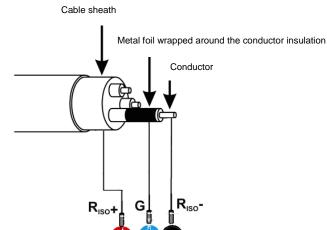
The same shall apply when measuring the resistance between two conductors of the cable, attaching to **G** terminal other conductors that do not take part in the measurement.
