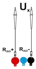
Connect the meter to a voltage source.
