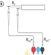
Connect test leads according to the drawing.
