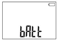
The battery pack is fully discharged, all measurements are blocked.
