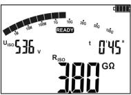
After the measurement is completed or stopped, read the result. The results of all completed measurements will be displayed (even when the measurement was interrupted)
