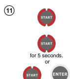
Press and hold **START** push-button. The measurement is performed continuously until you release the button or the pre-set time is reached.
