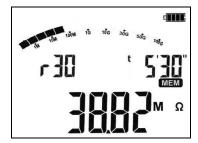
Resistance R<sub>ISO</sub> value, measured in time t=5'30'. Symbol r 🖺 indicates the selected time interval, in which the resistance value was recorded.
