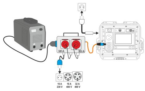
(3c) Measurement with PAT-3F-PE adapter. Connecting a 3-phase 16 A appliance.
