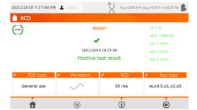
RCD must to be immediately switched on after RCD trips. Meanwhile the meter is powered from built-in rechargeable battery.
