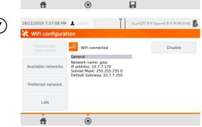
The network is saved and connection with the tester is established - connection's parameters are available.
