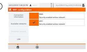
Pressing **Preferred network** enables displaying networks saved already in the tester. The network marked with is the network currently connected with the tester.
