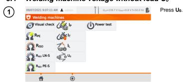
Before starting the measurement, similarly to sec.4.2, set  $U_0$  voltage, secondary voltage type, limit PEAK, limit RMS and optionally also the criterion of  $\pm 15\%$  PEAK.
