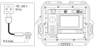
The device is powered from mains 195...265 V, 50 Hz.
