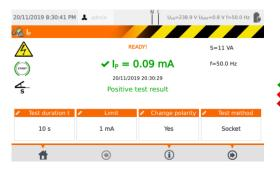
Positive test result: I<sub>P</sub> ≤ LIMIT
