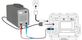
(2b) Variant with powering the welding machine directly from the mains socket.
