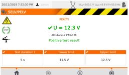
Positive test result: LOWER LIMIT ≤ U ≤ UPPER LIMIT
