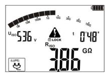
The meter measures the insulation resistance for selected pairs of leads in the following order: L-N, L-PE, N-PE.
