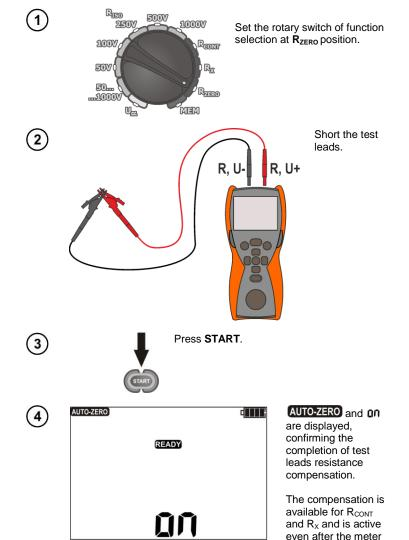
In order to remove the compensation made (and return to default calibration), perform the above-mentioned activities with test leads open – messages AUTO-ZERO and ON disappear, the following message is displayed OFF.
