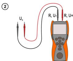
Connect the meter to a voltage source.
