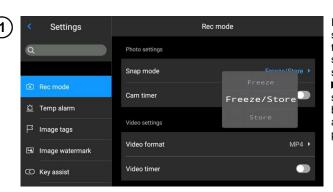
In the Real-time Image state, press the trigger button [5] to freeze the current scene, take images and save. Go to **Settings** ► **Shoot mode** and directly set the function of trigger button as image taking, thus achieving one-button taking pictures.
