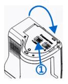
Close the lid and lock it with the latch (1). The card is now removed.
