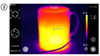
Press the trigger button. The image gets frozen as shown in the figure.
