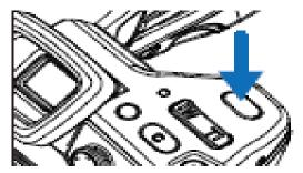
Long press the trigger button to start recording. Press the button briefly to stop recording and save the file.
